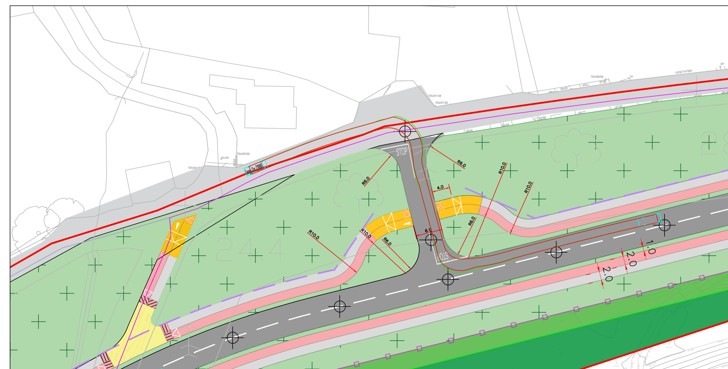
EXISTING ROAD SWEEP PATH - LARGE CAR
