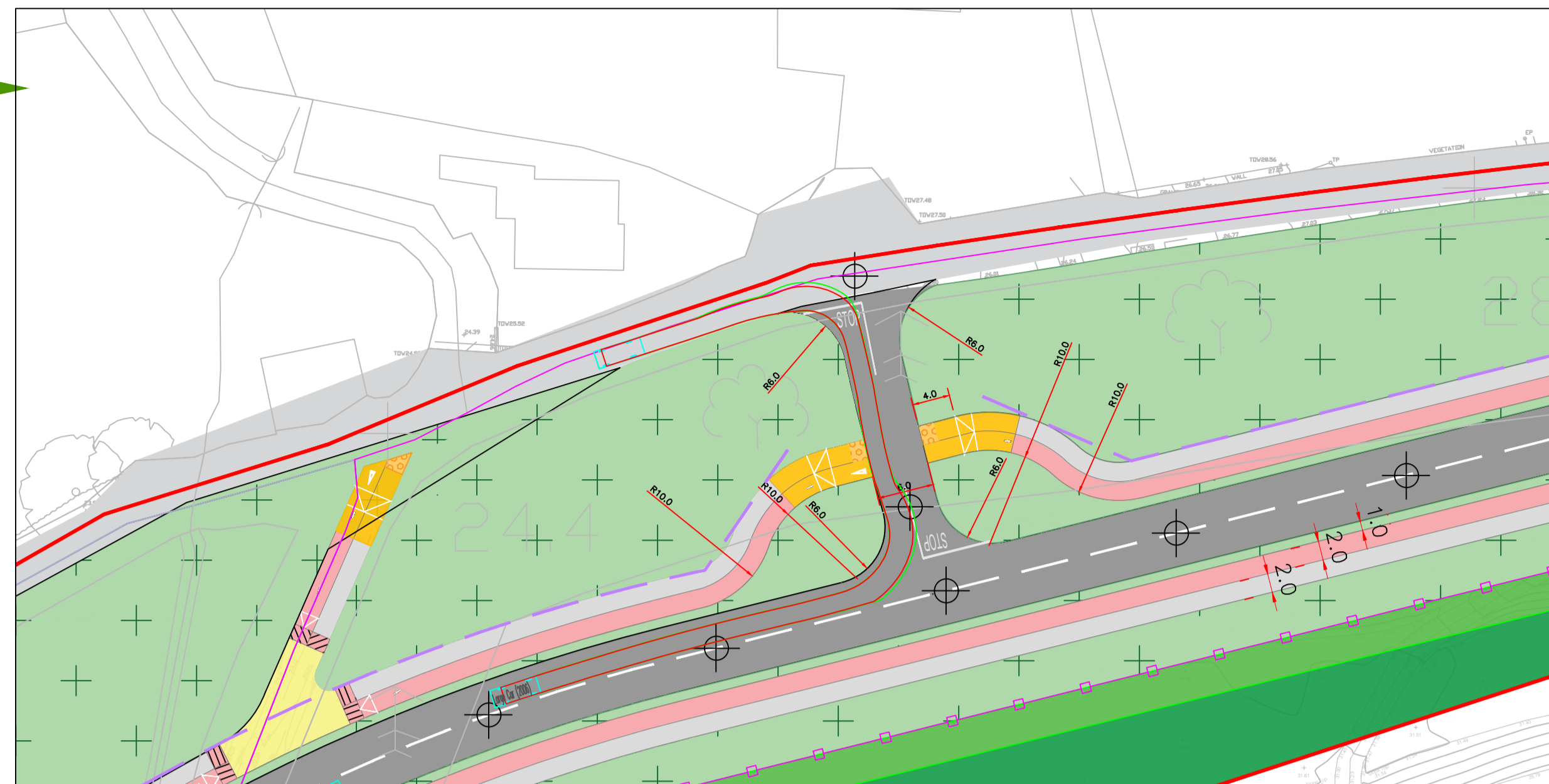
EXISTING ROAD SWEEP PATH - FIRE TRUCK
