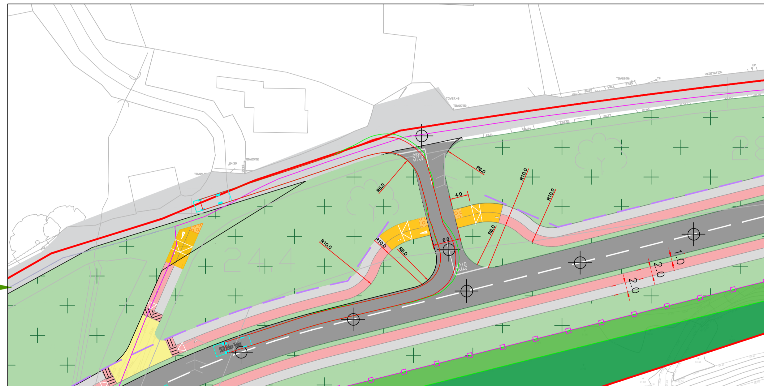
EXISTING ROAD SWEEP PATH - REFUSE VEHICLE
