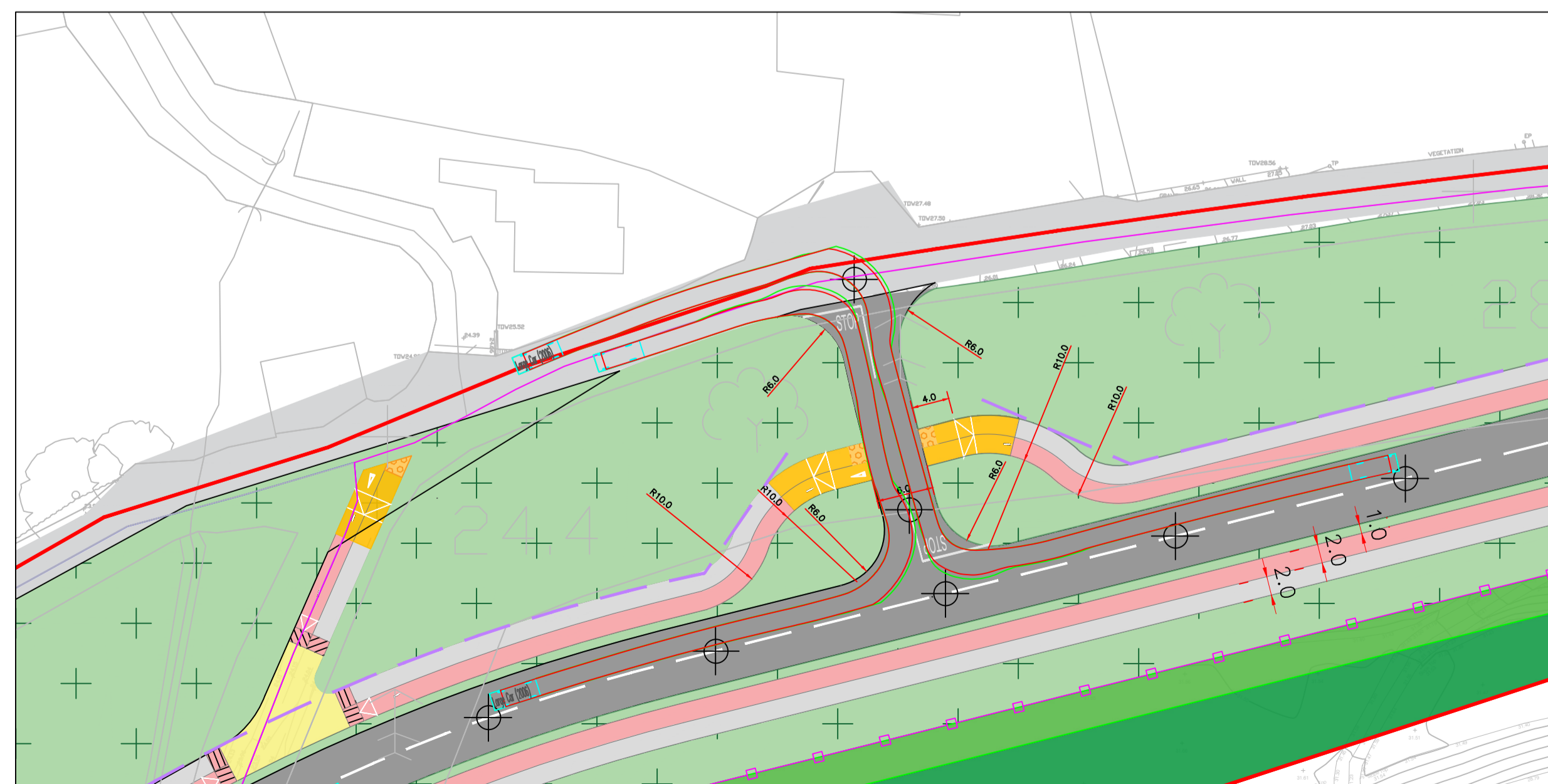
EXISTING ROAD SWEEP PATH - LARGE CAR
